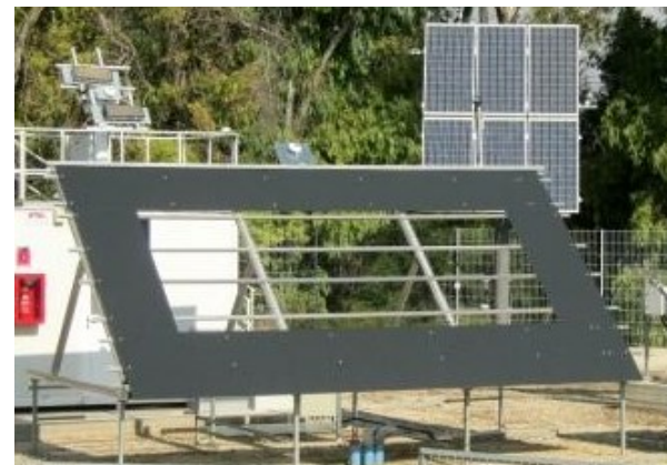
NOCT measurements (IEC 61215 Clause 10.5)
